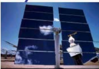
Heliostat Collector Panels
